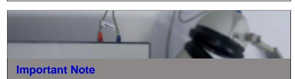
Once a headset has been selected and calibrated with its specific Audiometer they must always remain with the same audiometer. To ensure the headset remains with the same audiometer tag the headset with the specific audiometer serial number.
